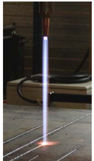
Strong cutting oxygen stream from a divergent nozzle: Photo taken from KOIKE in-house performance test. Nozzle tip at 275 mm above the plate, nozzle 106-D7#0
