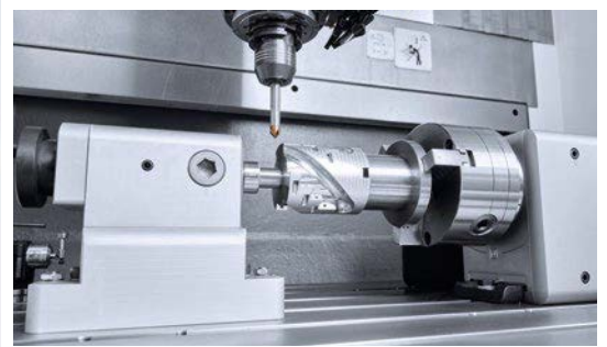
SIEMENS 828D control JobShop Package 4th axis including tailstock
