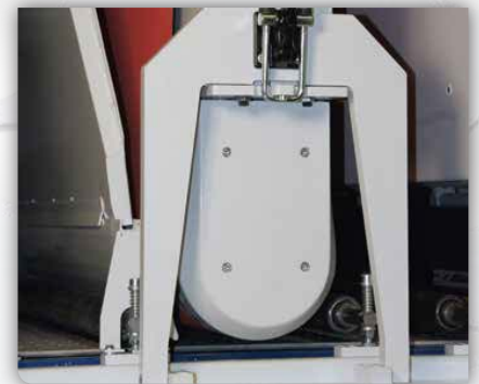
Rubber-coated grinding rollers for surface finishing and deburring.
